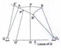
The mechanism is displaced as shown by the dotted lines in Fig. the point Q will trace out an approximately straight line.
