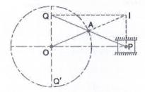
A is the middle point of PQ and OA = AP = AQ. The instantaneous centre for the link PAQ lies at I in OA produced and is such that IP is perpendicular to OP. Join IQ. Then Q moves along the perpendicular to IQ.
