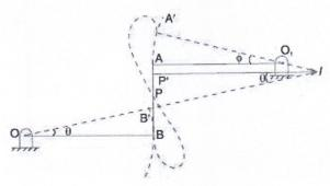
In Fig.  $OBAO_1$  is a crossed four bar chain in which O and  $O_1$  are fixed. In the mean position of the mechanism, links OB and  $O_1A$  are parallel and the coupling rod AB is perpendicular to  $O_1A$  and OB. The tracing point P traces out an approximate straight line over certain positions of its movement, if  $PB/PA = O_1A/OB$ .
