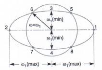
1. For one complete revolution of the driven shaft, there are two points i.e. at  $0^{\circ}$  and  $180^{\circ}$  as shown by points 1 and 2 in Fig. where the speed of the driven shaft is maximum and there are two points i.e. at  $90^{\circ}$  and  $270^{\circ}$  as shown by point 3 and 4 where the speed of the driven shaft is minimum.
