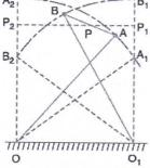
The point P, which is the mid-point of AB traces out an approximately straight line parallel to  $OO_1$ . The proportions of the links are, usually, such that point P is exactly above O or  $O_1$  in the extreme positions of the mechanism i.e. when BA lies along OA or when BA lies along OA or when AB lies along AB
