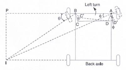
In Ackerman steering gear, the mechanism *ABCD* is a four bar crank chain, as shown in Fig.
