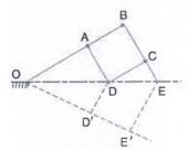
It consists of a jointed parallelogram ABCD as shown FIG. It is made up of bars connected by turning pairs. The bars BA and BC are extended to O and E respectively, such that
