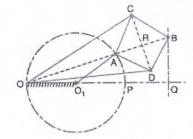
It may be proved that the product  $OA \times OB$  remains constant, when the link  $O_1A$  rotates. Join CD to bisect AB at R. Now from right angled triangles ORC and BRC, we have
