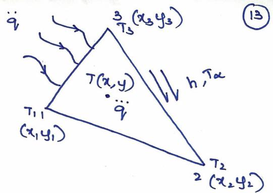
Calculate the shape functions, conductivity matrix, thermal load vector and temp values at the nodal points of a triangular element as shown in fig.  $t = 10\text{mm}$ ,  $K_x = K_y = 50\text{W/mK}$
