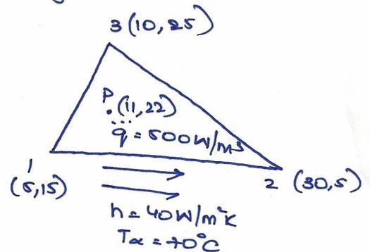
$$\{P_T\} = \frac{\ddot{q}_T A t}{3} \begin{bmatrix} 1 \\ 1 \\ 1 \end{bmatrix} = \frac{500 \times 150 \times 10}{3 \times 10^6 \times 10^3} \begin{bmatrix} 1 \\ 1 \\ 1 \end{bmatrix} \quad [A, t \text{ are in mm}]$$
