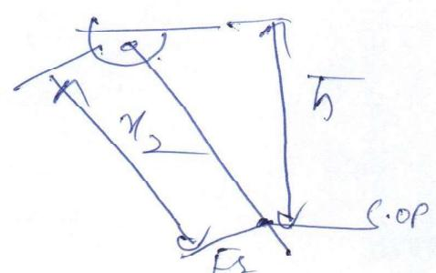
$$b = \frac{\bar{x} + \frac{I_y}{A} \sin^2 \theta}{\bar{x}} = \frac{1.25 + \left( \frac{1 \times 5^3}{12} \right) (\sin 30)^2}{5 \times 1 \times 1.25} = \underline{\underline{1.667 \text{ m}}}$$
