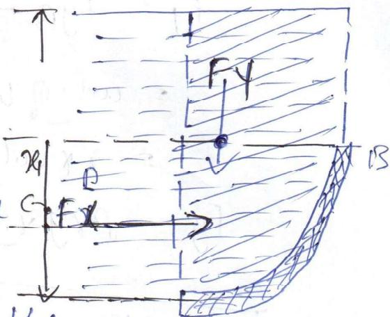
$F_y$  = vertical hydrostatic pressure force
