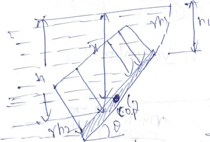
$$\bar{h} = \bar{x} + \left( \frac{J_G \sin^2 \theta}{C_G - \bar{x}} \right)$$
