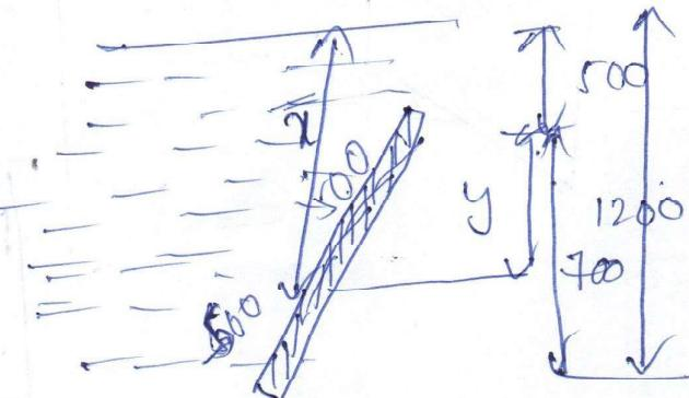
$$F = \gamma A \bar{x}, \bar{h} = \bar{x} + \left( \frac{\gamma g \cdot \sin^2 \theta}{A \cdot \bar{x}} \right)$$
